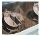
Mixes in half the time. Twin flighting double augers have 4 pickup points (2 on each auger).
