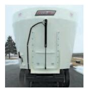
Optional large rear door for fast unloading of pre-mix loads.
