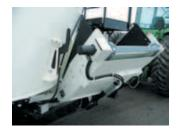
Simple chain and slat conveyor can be assembled for right or left hand discharge. Hydraulically controlled conveyor extension for feeding on the floor or in feed bunks.
