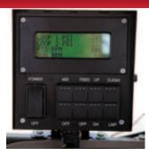
Complete control from the tractor cab monitor for mix, feed and cleanout modes.
